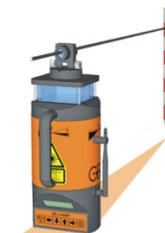
**Please note:** Before starting work, especially on steep slopes, check or adjust the inclination and inclination assignment via fixed points or by surveying.
