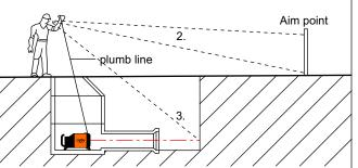
. Set up laser over the axis.
