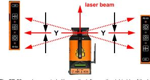
The FE-53 can be mounted either on the left or on the right side of the laser. Because of reasons of functionality, the keyboards of both devices must be on the same side.
